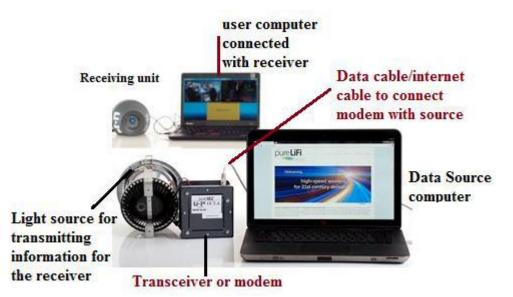
The input data from the source computer is converted to bits, zeros and ones, to represent as digital signal. Depending on this stream of digital ones and zeros data, the high illuminated LED bulb ON-OFF condition is controlled with the help of driver circuit. This highly flickered LED light is transmitted to the nearby receiver, photodiode. This weak received signal
